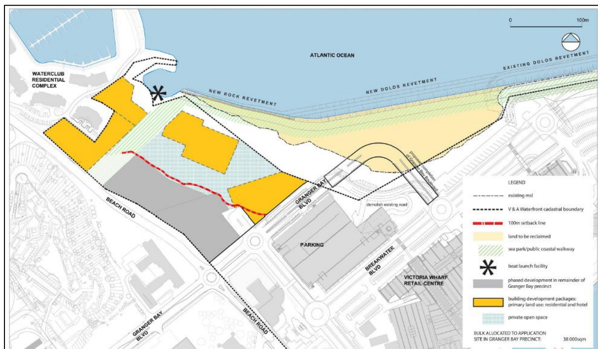
Figure 2: Approved 2019 Granger Bay notional precinct development comprising dolos revetment with land reclamation and mixed-use development.
